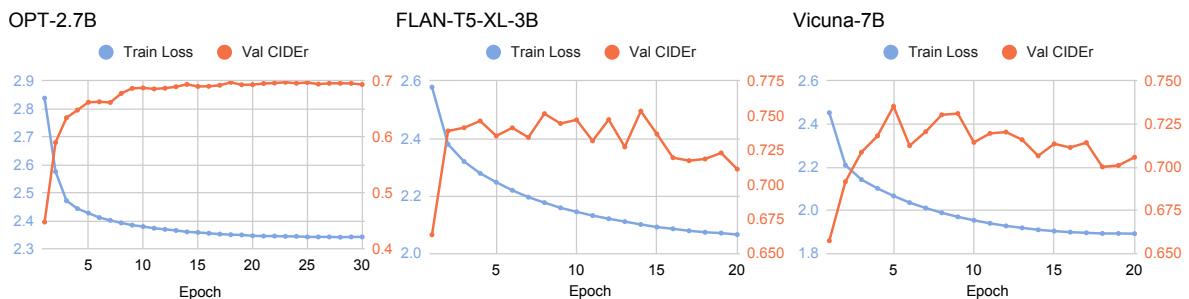
Figure 5: Training curves of a video captioning model with different sizes of LLMs. (a), (b), and (c) show training curves of LLMs with sizes 2.7B, 3B, and 7B respectively.
